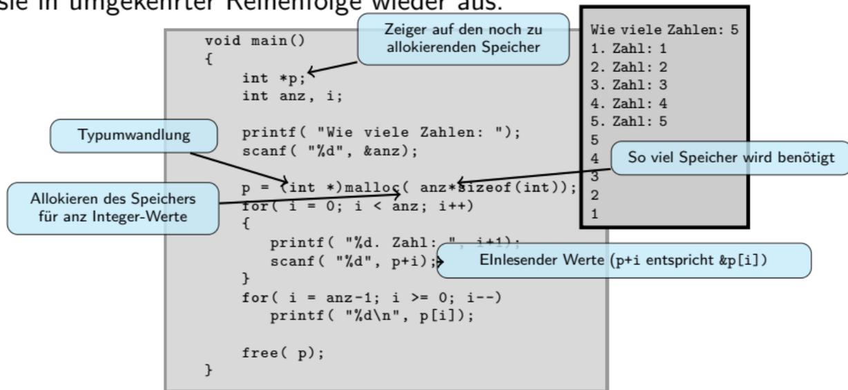
The diagram illustrates the execution of a C program that dynamically allocates memory for an array of integers. The code is shown in a grey box, and a terminal window on the right shows the user's input and the program's output. Annotations in blue boxes explain key parts of the code and the user's interaction.
