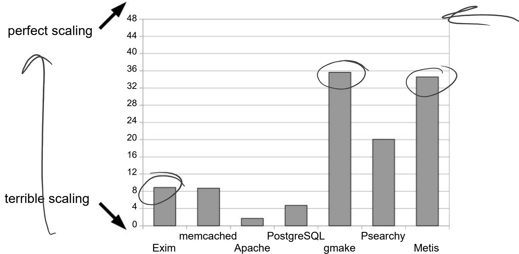
Y-axis: (throughput with 48 cores) / (throughput with one core)
